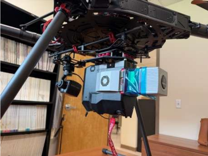
Multispectral imager and Lidar on Alta-X drone
